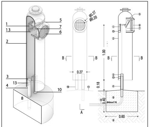
**The lighting and furniture elements are designed and custom built with waste** such as discarded divers' oxygen bottles. Care for the environmental impact is also perceived in the orientation of the lamp so that it avoids light pollution, as well as in the watering of the greenery, which is supplied with recycled water.
